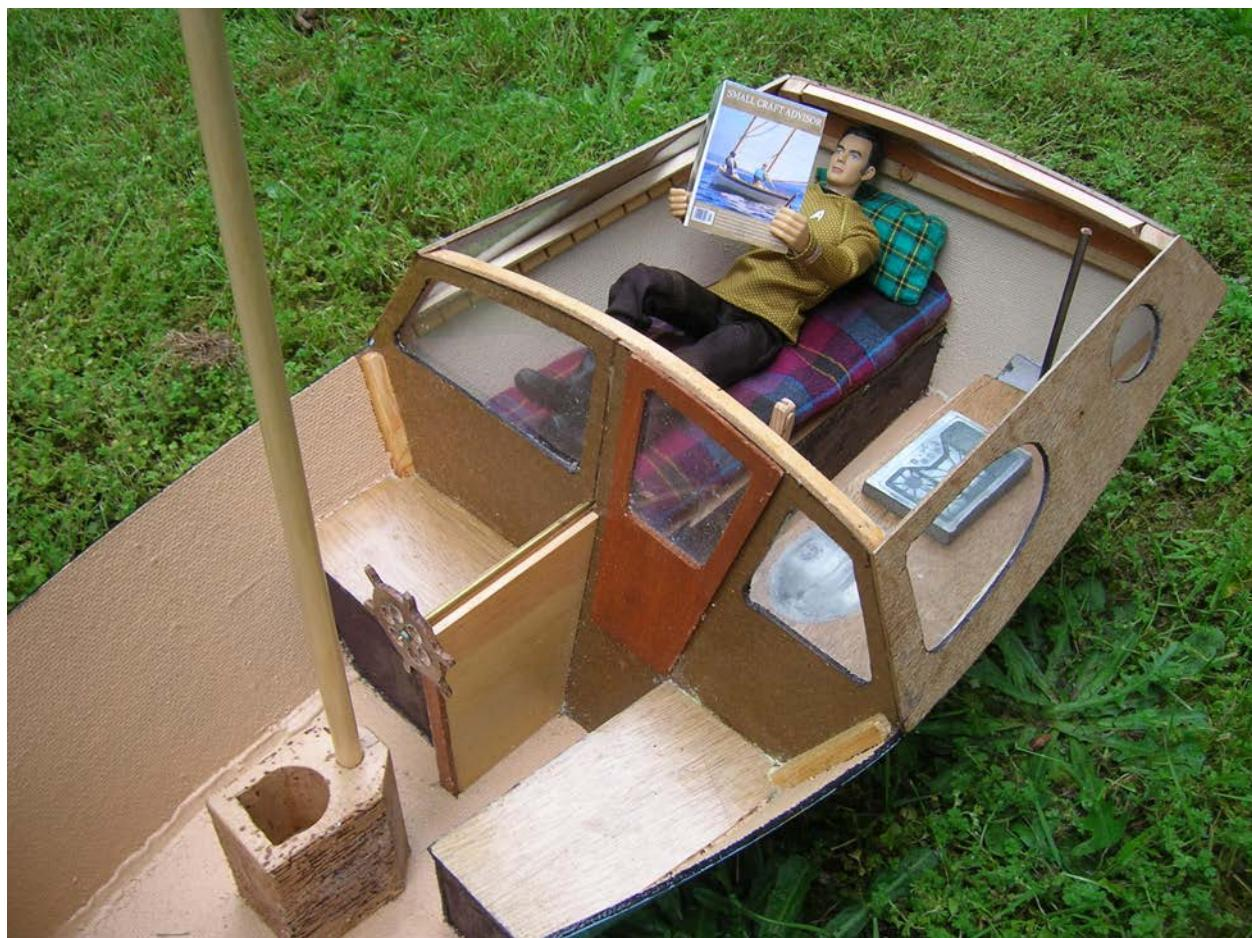
By installing oar locks, the vessel can be rowed by sitting on the bow locker and using the outboard well for a foot rest.
