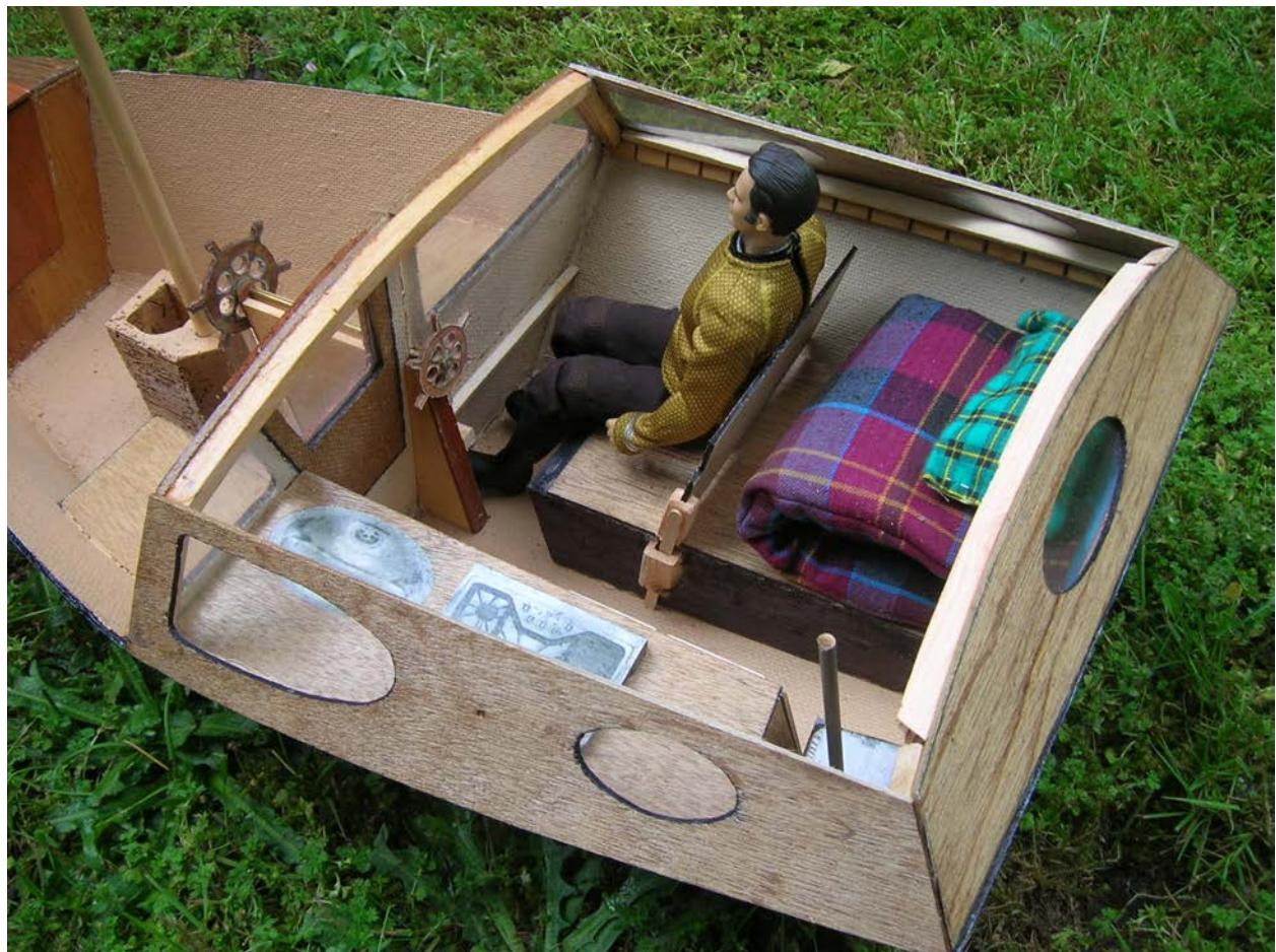
The forward 18" panel of the bunk lifts out creating a foot well. The panel is then installed in supports to form the back of the helmsman's seat. A narrow shelf supported by the CB trunk and hull sides should be installed under the forward window for compass, VHF etc.
