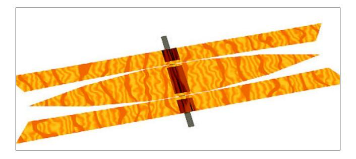
There should be piece of duct tape under the panels, full width. The tape will act as a hinge.
