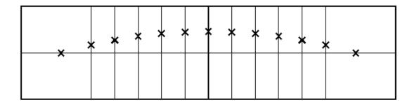
All the points for one side of the bottom panel are now on the plywood and all that is left to do is to scribe a nice smooth curve passing through all those points.
