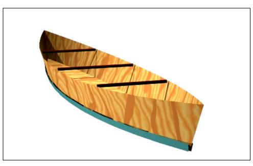
This ends the assembly phase. The next step is the fiberglass work.
