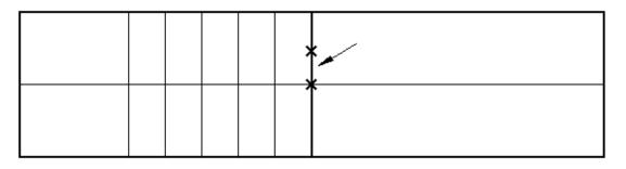
The second point is on the first line (at 12" from the edge) and the distance above the centerline is 273 mm. Mark it.
