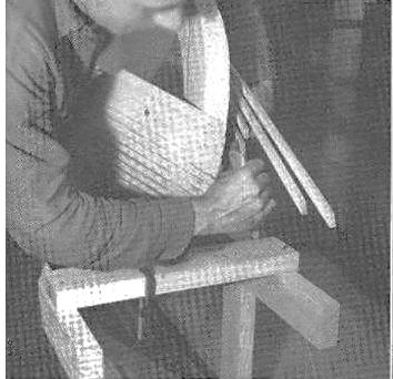
Bevel strips so they meet in front of stem. A tight fit is not necessary, since the stems are covered with two layers of cloth and resin.
