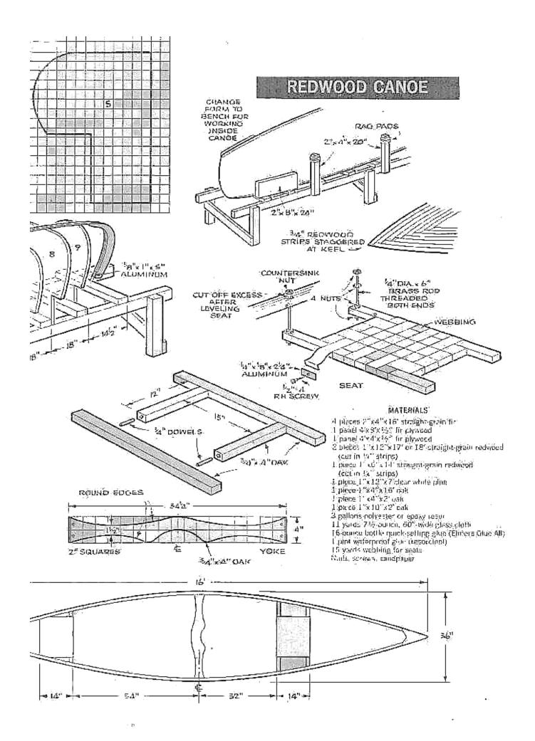
When all strips are in place, sand the bull and give the outside a coat of polyester or epoxy resin. When this has set, make a thin-point nail set and punch all nails in each strip through, into the form.
