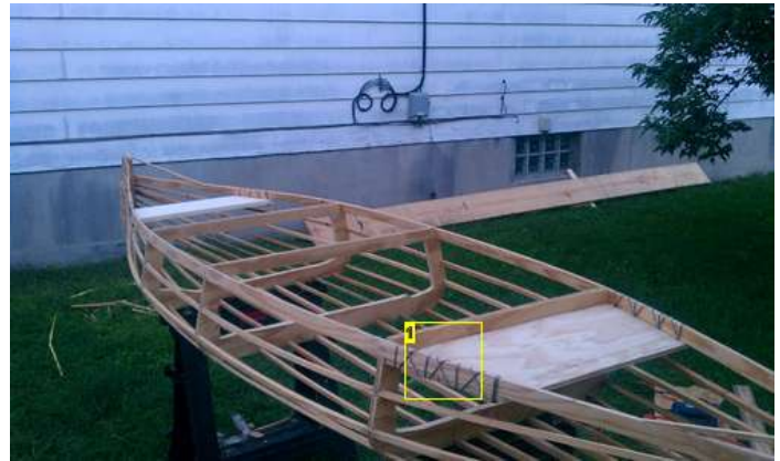
Image Notes 1. Seats are lashed in place. If sealed against water, paracord is a good option here.
